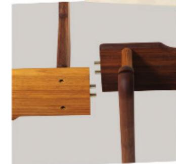
Align the long legs so as the steel bolts can pass through the holes.
