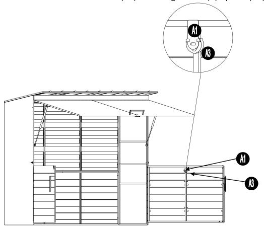
Place remote control (A1) onto remote control holder (A3).
