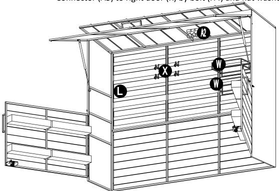
Place the big rack (W) and the small rack (X) on the Back Decorative Panel (L), magnetic suction lamp (A2) onto the middle roof (B).
