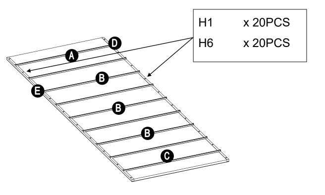
Attach side panel (D/E) to roof (A/B/C/F) by bolt (H1) and washer (H6).
