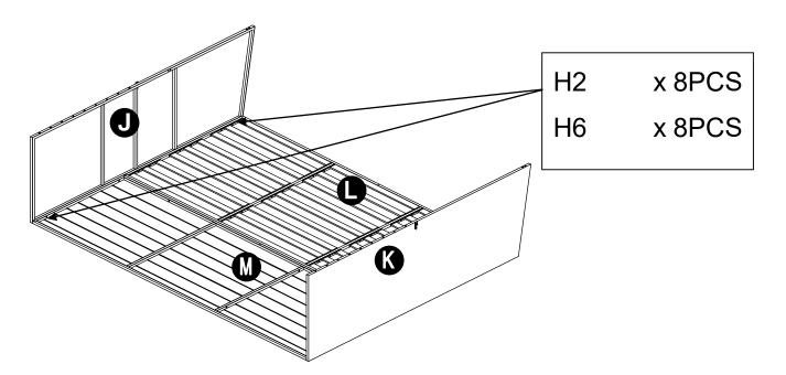
Attach left/right side panel (J/K) to upper/lower panel (L/M) by bolt (H2) and washer (H6).
