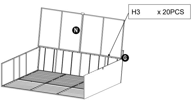
Attach door (N) to beam (G) by bolts (H3).
