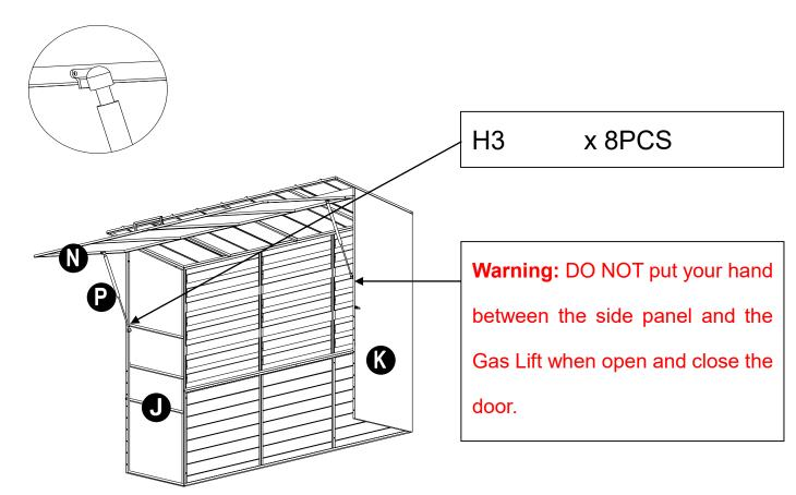
Attach Gas Lift (P) to the Flip Door (N), the left side panel (J) and the right side panel (K) by Bolt (H3).
