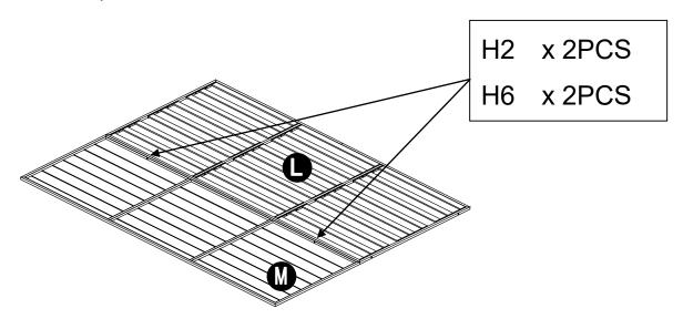
Attach upper panel (L) to lower panel (M) by bolt (H2) and washer (H6).
