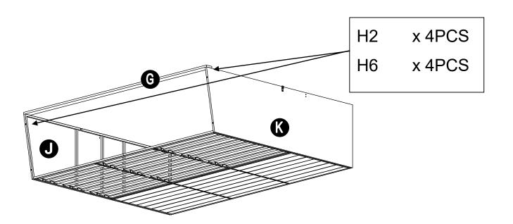
Attach beam (G)to left/right side panel (J/K) by bolt (H2) and washer (H6).
