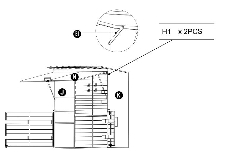
Attach the support bar (B1) to the L/R side panel (J/K) with bolt (H1)
