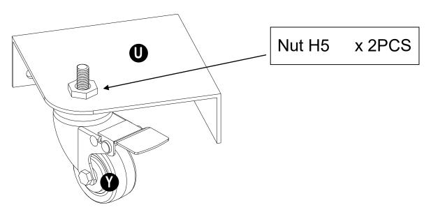
Attach L/R Universal wheel (Y) to the L/R connector (U/A5), lock them by Nut (H5).
