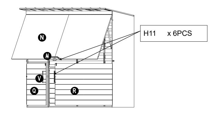
Attach the L/R right Doorknob V to the L/R Door (Q/R), attach Doorknob (A4) to the door (N) by Bolt (H11).
