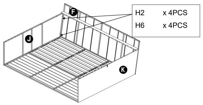
Attach roof (F) to left/right side panel (J/K) by bolt (H2) and washer (H6).
