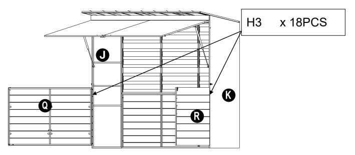
Attach the hinge at the left door (Q) and the right door (R) to the left side panel (J) and the right side panel (K) by Bolt (H3) and lock them.
