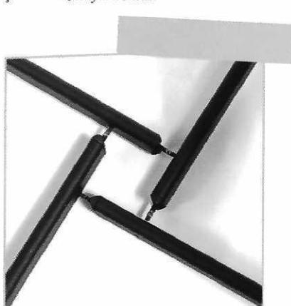
When a square is formed as in the picture below, place the screws and tighten.
