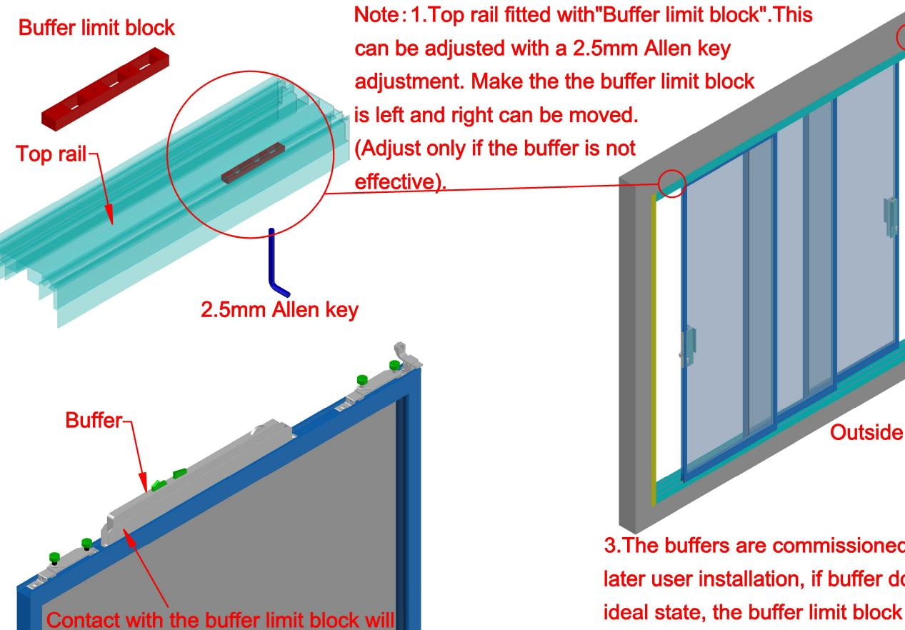
3.The buffers are commissioned at the factory.In the later user installation, if buffer does not reach the ideal state, the buffer limit block can be adjusted.
