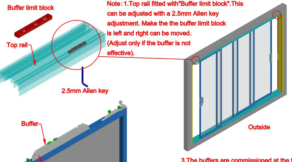
Contact with the buffer limit block will play a cushioning effect, to avoid the glass door vigorously colliding with the side frame.
